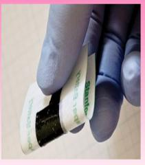
Afterwards scientists placed the double-layer films on both sides of regular paper. In such a construction the lithium films work as battery electrodes and the nanotube films play the role of current collectors. The role of electrode separator is played by the paper, which is also used as a mechanical support.
